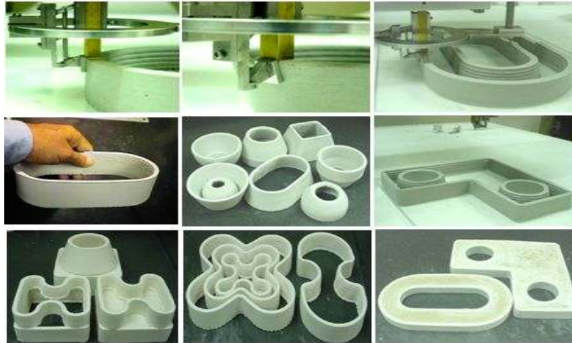
Figure 2: CC in Operation (First Row) and Representative 2.5D and 3D Concrete Shapes
