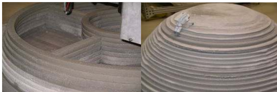
Figure 4: Dome Structures Built using CC at NASA Marshall Space Flight Center
