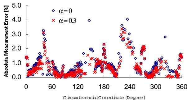
Figure 4: Measurement Errors of an Aluminum Frame for  $\alpha = 0$  and 0.3
