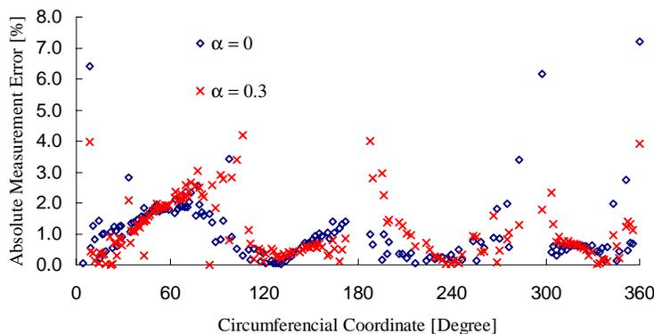
Figure 6: Measurement Errors of a Rectangular Room for  $\alpha = 0$  and 0.3
