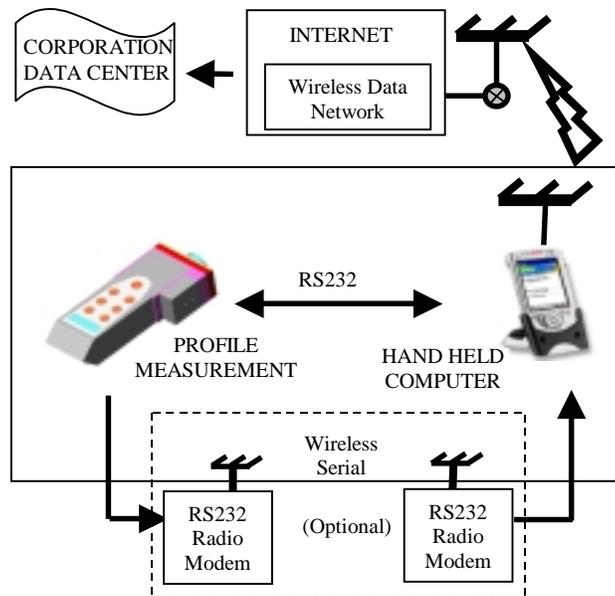
**Figure 2: Schematic of Wireless Communication with Laser-Based Measurement System**
