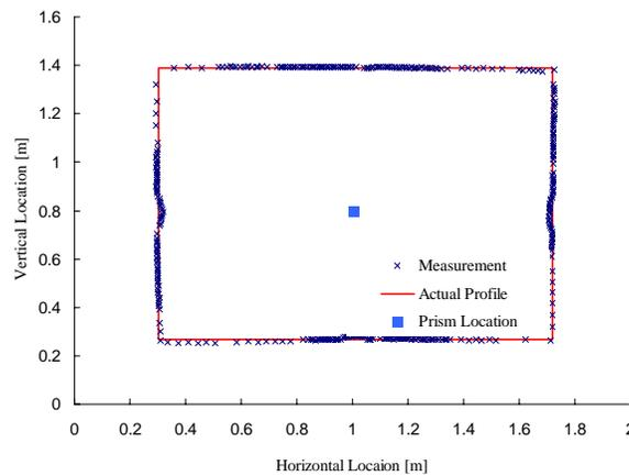
Figure 3: Measurement of an Aluminum Rectangular Frame at 1 RPM
