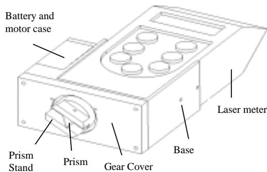
**Figure 1: Schematic of Laser-Based Full Profile Measurement System**
