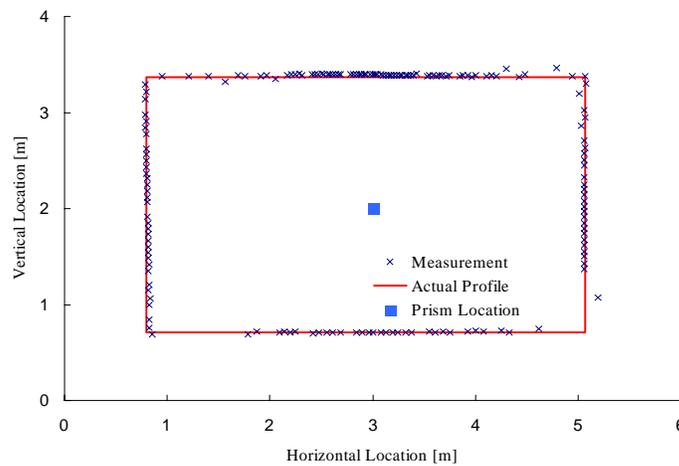
Figure 5: Measurement of a Rectangular Room
