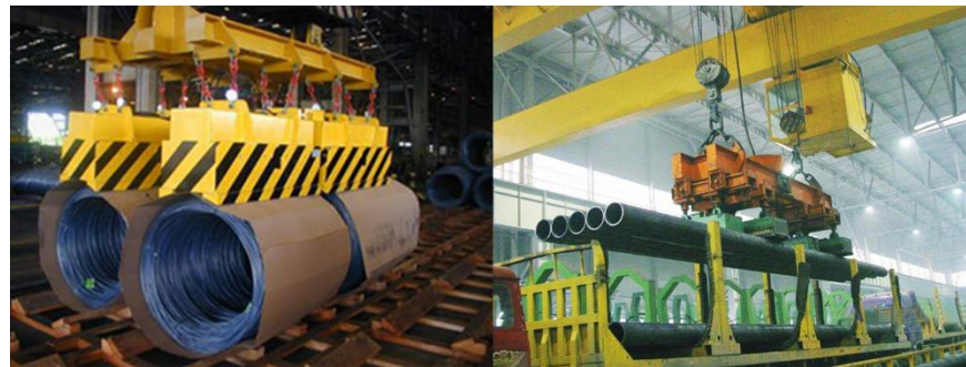
Fig. 6. Overhead crane with electromagnetic beam will be simulated in the triquetrous of MMCT.
