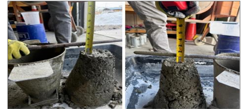
Fig. 2. (a) Slump test results, (b) Slump measurements
