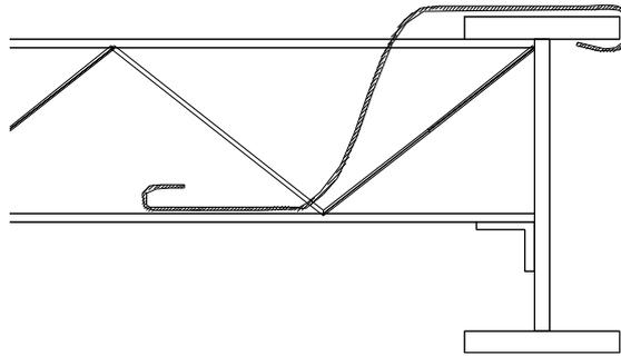
Figure 3. Hook steel bars in end. Lateral beam support is designed by rigid joint.
