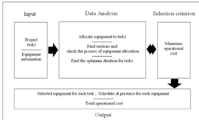
**Figure 3: Equipment Selection Process and Analysis**
