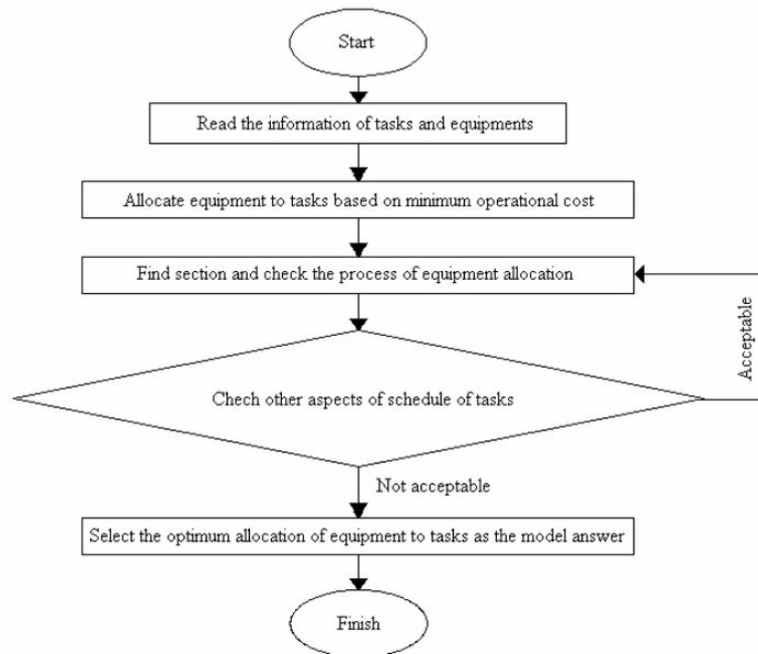
**Figure 5: Flow Chart of the Equipment Matching**
