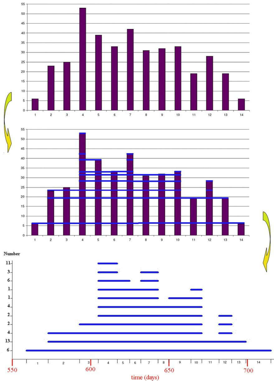
**Figure 10: Process of Developing a Diagram of Schedule of a Machine**
