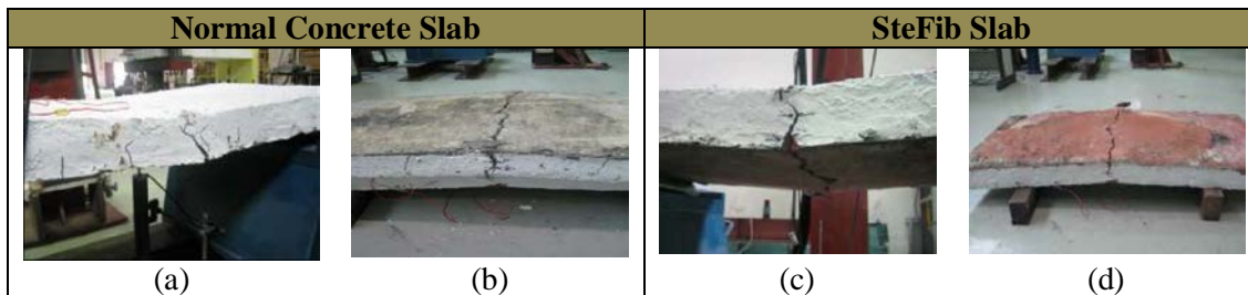
Figure 7: Crack Pattern on Slab Panel
