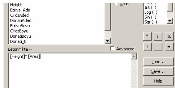
Figure 6: Computation of Concrete Amount
