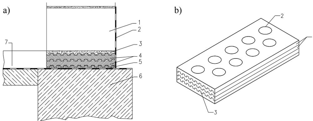
**Figure 3: Insulating Block; 1 - Masonry, 2 - Water-proofing, 3 - Cement Mortar or Concrete, 4 - Insulating Block, 5 - Paste, 6 - Foundation, 7 - Floor**
