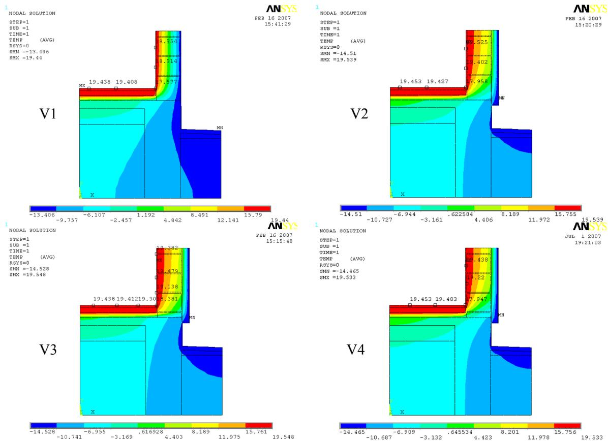
Figure 4: FEA Results - Distribution of Thermal Field for Solution V1 to V4
