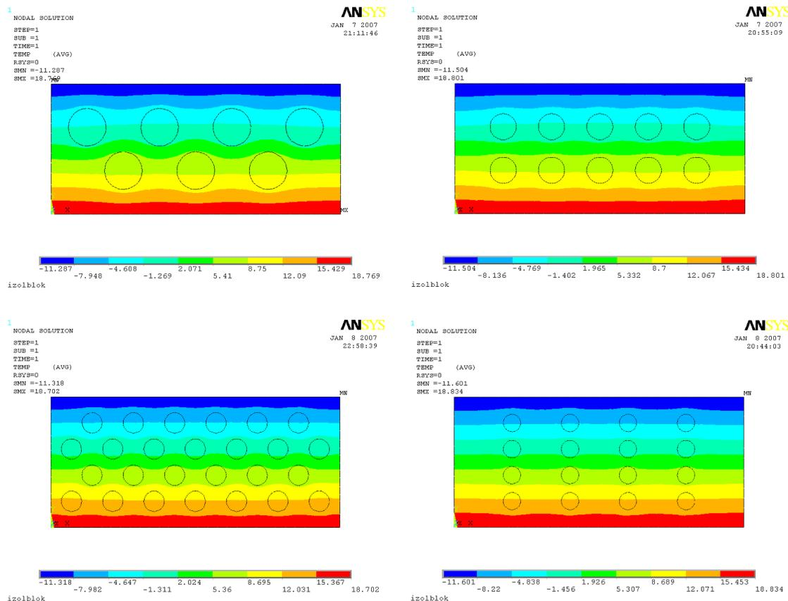
**Figure 5: FEA Results-Distribution of Thermal Field for Different Size and Placement of Openings**
