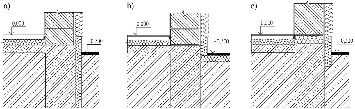
**Figure 2: Wall Footing Detail - Interruption of Thermal Bridge, Methods of Solution**
