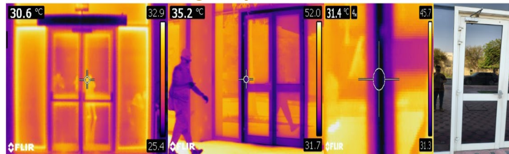
Figure 3 : IR and normal images capturing the emergency exit doors of ESB building showing signs of thermal leakage and upon visual and physical inspection leakage detected.
