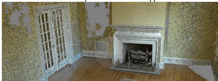
Figure 4: Point cloud generated within Agisoft Photoscan, with informational gaps present along uniform surfaces
