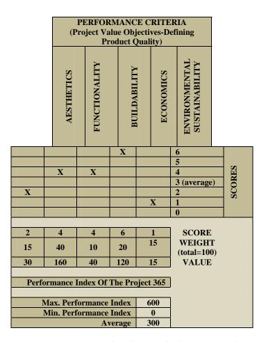
Figure 1: Example of an Output Objectives Matrix
