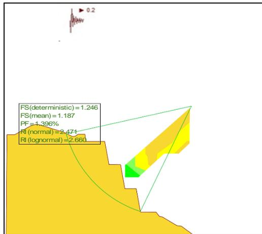
**Fig.5** Slope profile modeling in Slide
