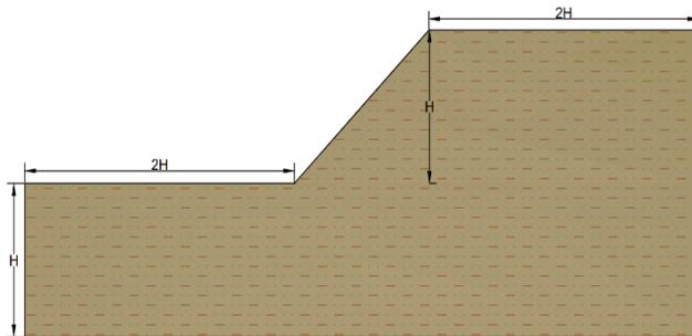
**Fig. 2.** Scheme of boundary conditions for synthetic slopes
