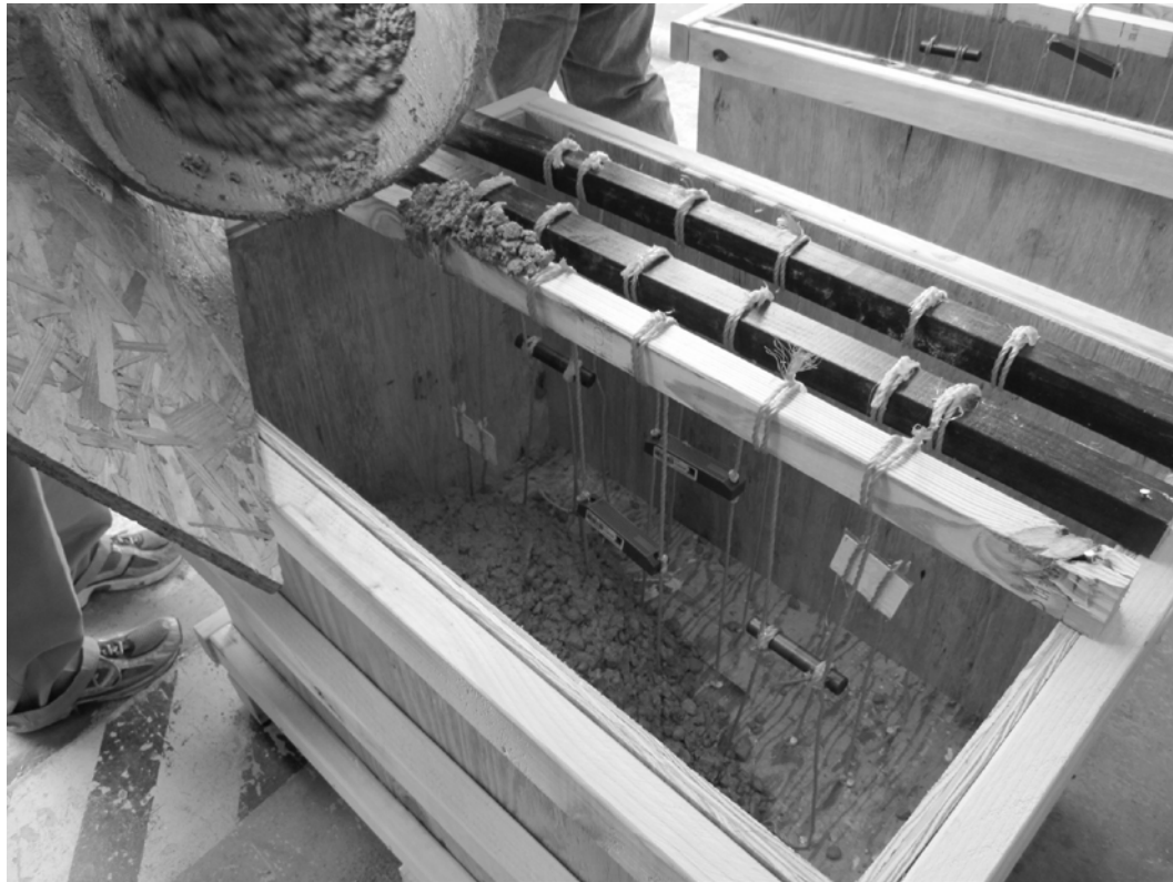
Figure 2. RFID tags placed in the form
