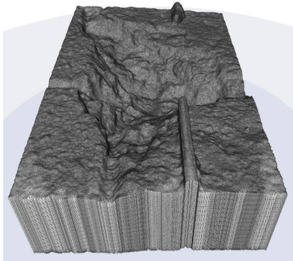
*Figure 3 Typical spall damage presented in 3D computer model*
