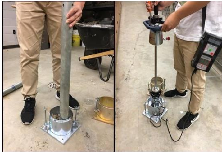
(a) Proctor Compaction (b) LWD Test in Mold Fig. 4. Photos of laboratory LWD testing
