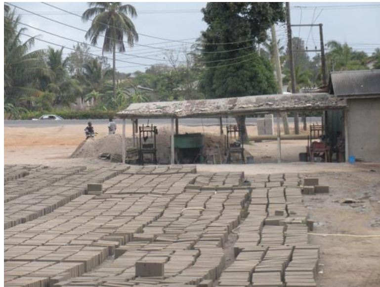
Figure 3. Masonry units drying in the sun in Tanzania (photo by Dr. James Pocock)
