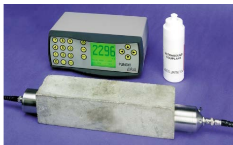
Figure 1: Pundit tester for ultrasonic pulse velocity
