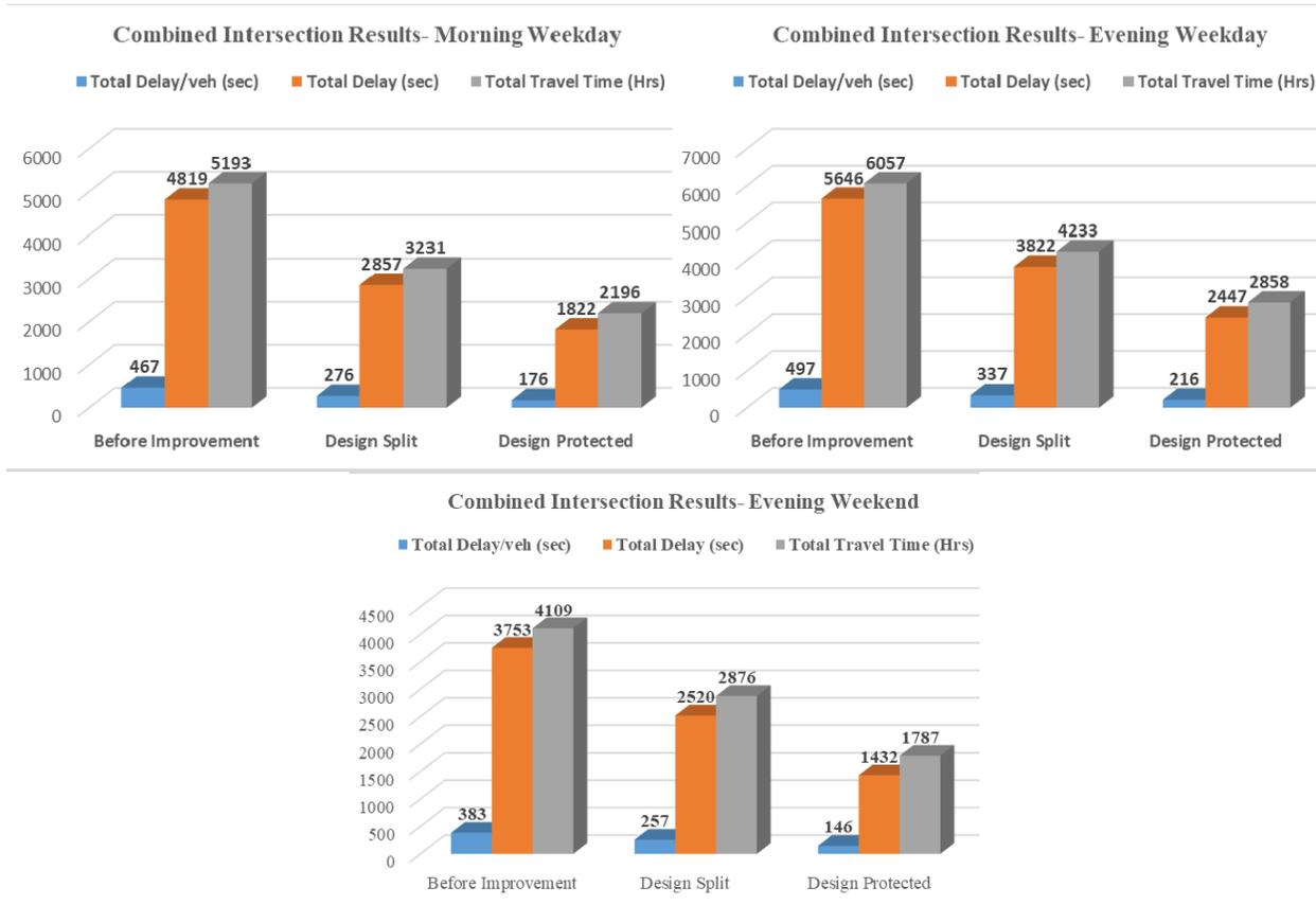
**Fig 3.** Intersection combined results of total delay/veh (sec), total delay (sec), total travel time (hrs), (a) morning peak hours of weekday, (b) evening peak hours of weekday, and (c) evening peak hours of weekend.
