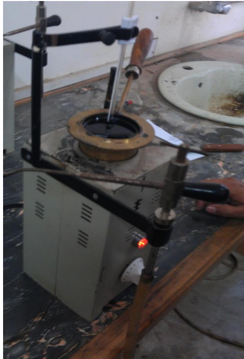
Figure 5: Apparatus for Determining Flash and Fire Point
