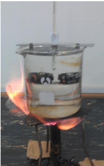
Figure 3: Apparatus for Determining Softening Point of Asphalt
