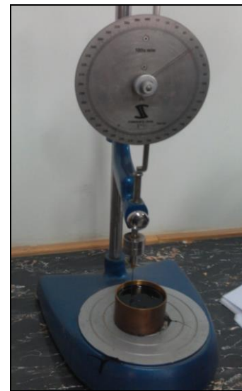
Figure 1: Apparatus for Bitumen Penetration Test
