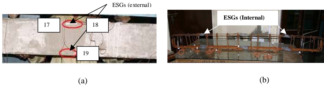
Figure 3: Installation of ESGs (a) On surface (b) On rebars embedded inside
