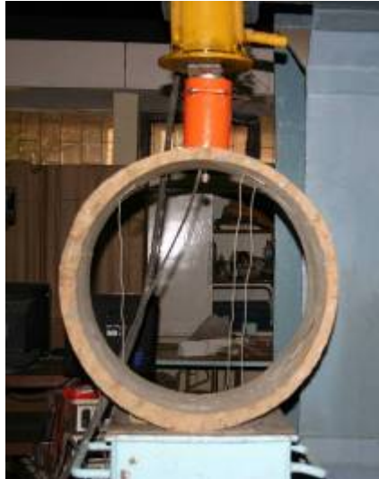
Figure 7: Monitoring of model tunnel lining using ESGs
