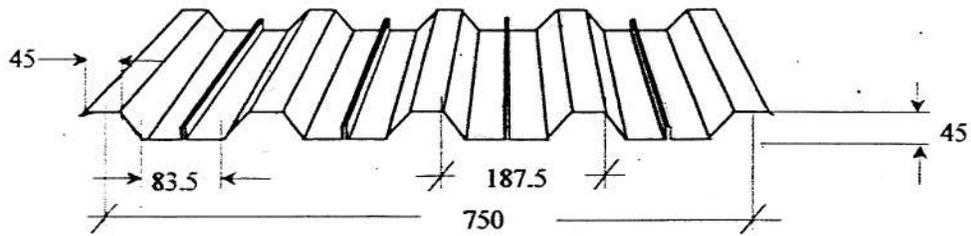
Figure 1: Cross Section of Peva 45 (units in mm)
