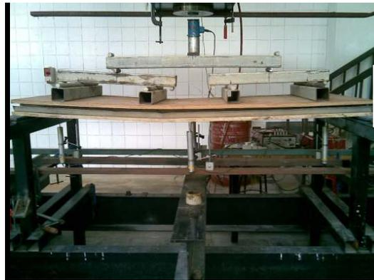
**Figure 6: The Panel Deflects Under Loading in the Laboratory**
