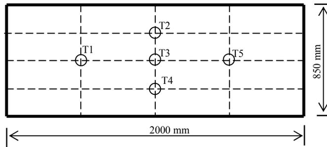
**Figure 5: Schematic Drawing of the Transducers Location**
