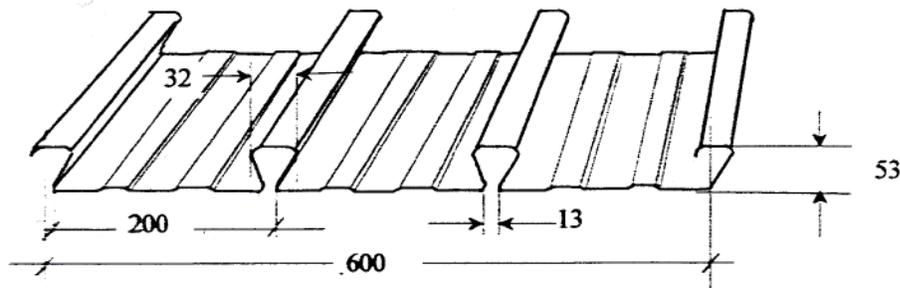
Figure 2: Cross Section of Bondek II (units in mm)
