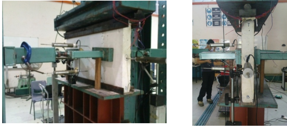
Figure 5: Final set-up of wall panel
