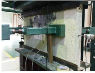
(c) Surface failure at the top wall panel
