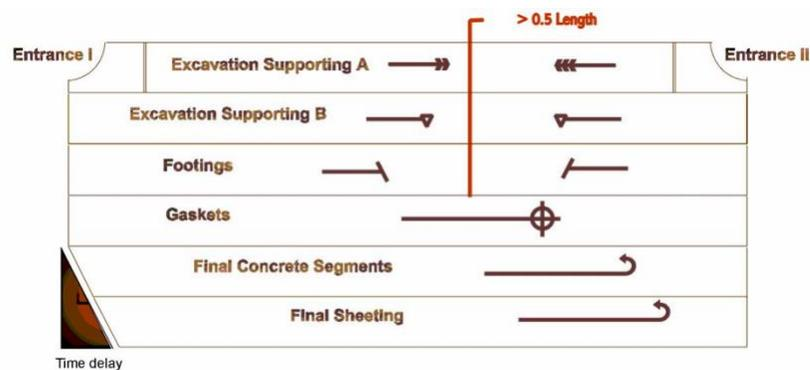
**Figure 8: Task Sequencing during Rapid Tunnel Excavation.**
