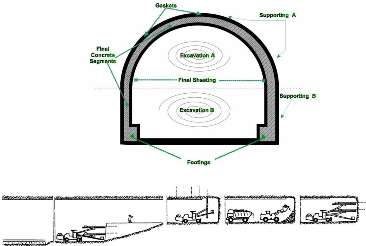
**Figure 5: Schematic Description of Tunnel Excavation Tasks (a) front view, (b) side view.**
