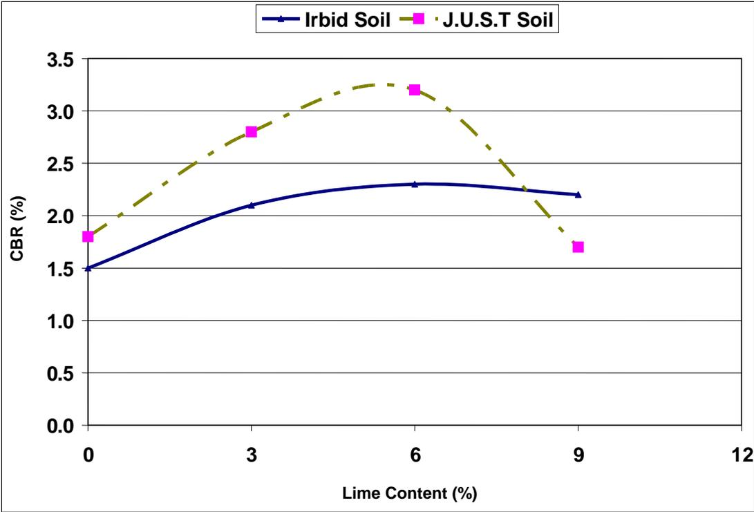
**Figure 5 Effect of Lime Content on California Bearing Ratio of Evaluated Soils**
