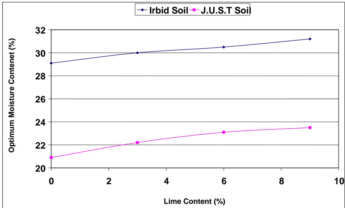
Figure 1 Soil Optimum Moisture Content at Different Contents of Hydrated lime
