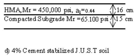
**Figure 9 Pavement Layers Thickness for Unstabilized soils, 6% Lime, and 4% Cement Stabilized Soils**
