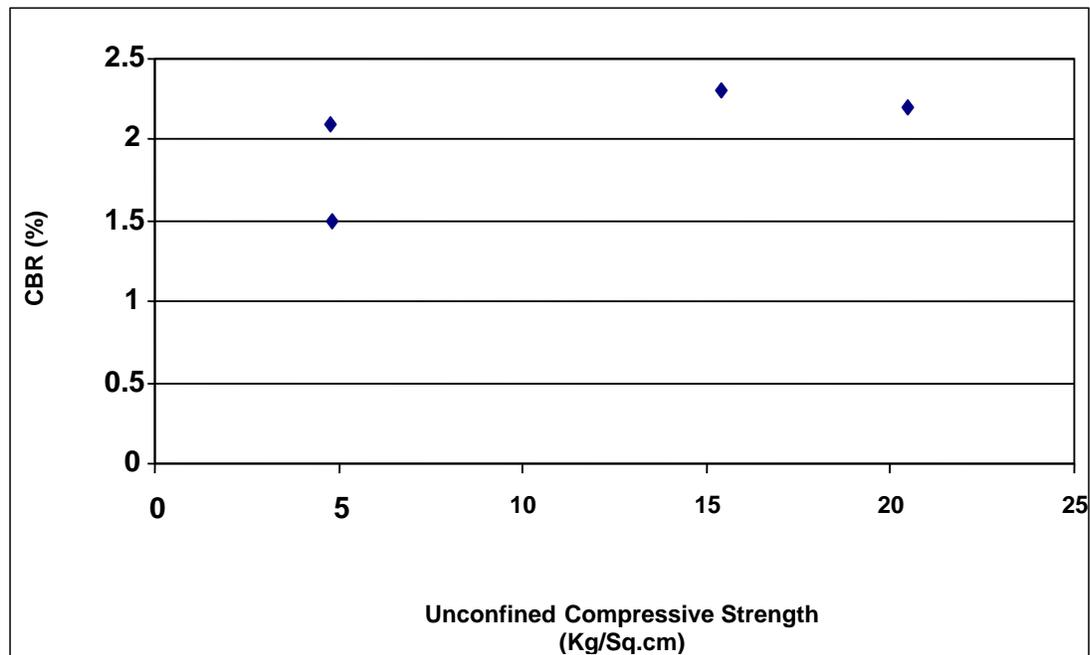
**Figure 8 Unconfined Compressive Strength Versus CBR for Irbid Soil**
