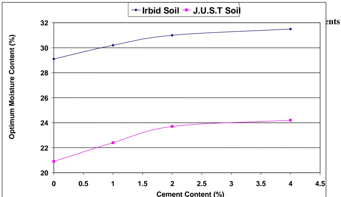
Figure 2 Soil of Optimum Moisture Content at Different Portland Cement Contents
