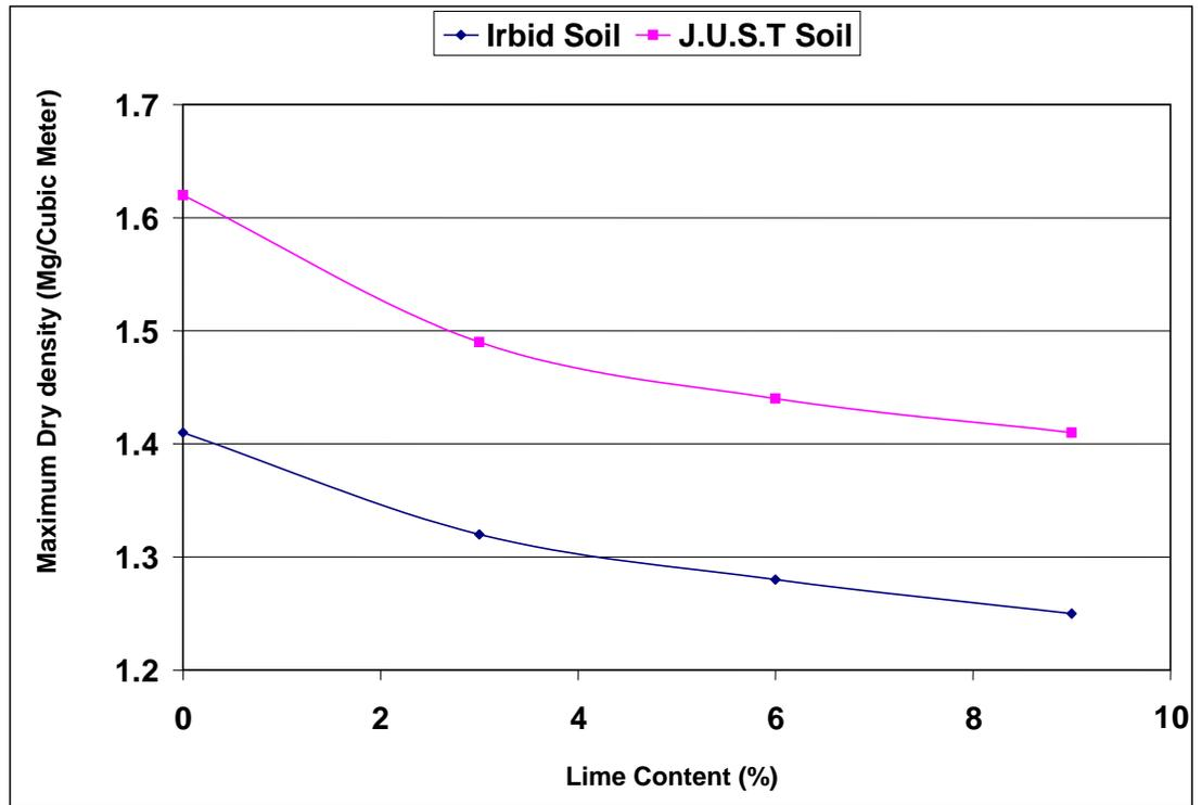
Figure 3 Maximum Dry Density of Soils Mixtures at Different Contents Lime
