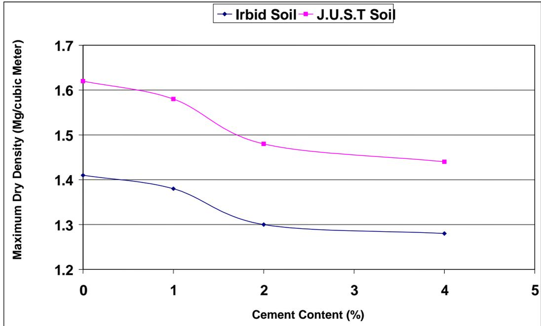
**Figure 4 Maximum Dry Density of Soils Mixtures at Different Content of Portland Cement**
