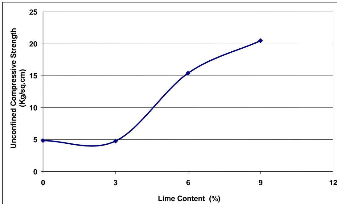
**Figure 7 Unconfined Compressive Strength of Irbid Soil at Different Percentages of Hydrated Lime (Alawneh, 1989)**
