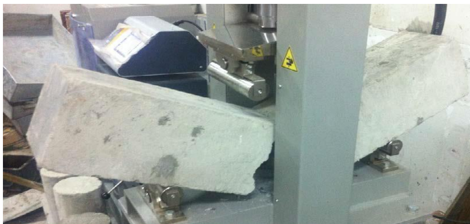
Figure 8 & 9: Samples under Flexural Loading
