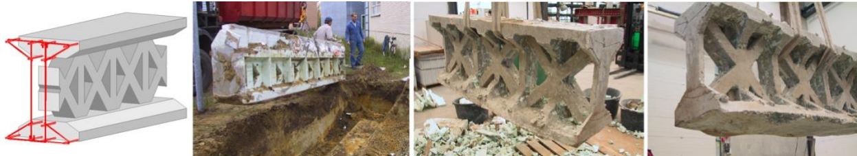
Figure 2: Outline of proposed foundation beam and result of dug up foundation of the pilot project
