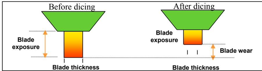
**Figure 2: Phenomenon of the Blade Before and After Dicing**
