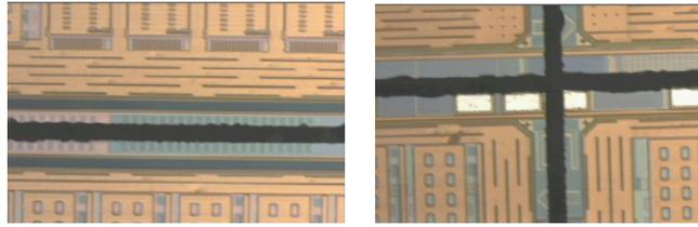
**Figure 1: Example of Saw Kerf Width on the Wafer**
