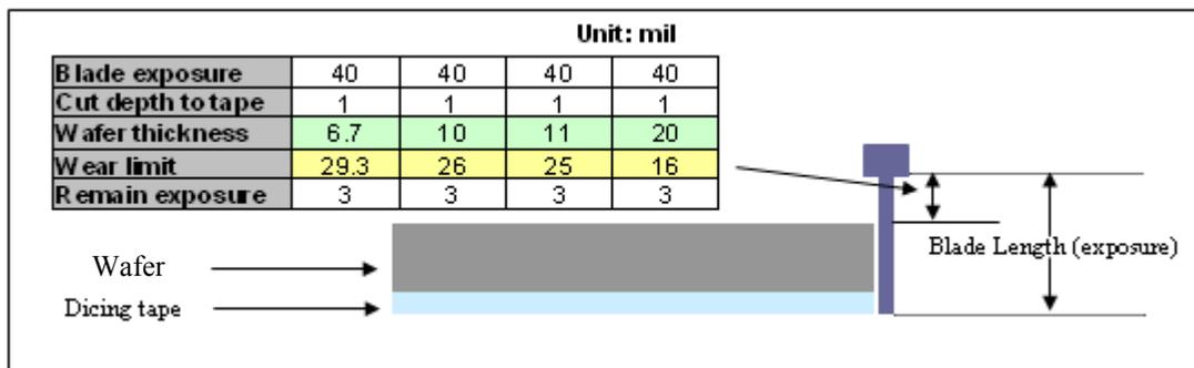
**Figure 3: Blade Length and Usable Length Calculation**
