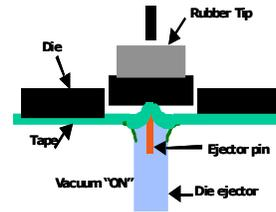
**Figure 5: Die Attach Pickup Process**
