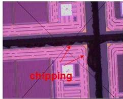
**Figure 4: Wafer Chipping Photo**
