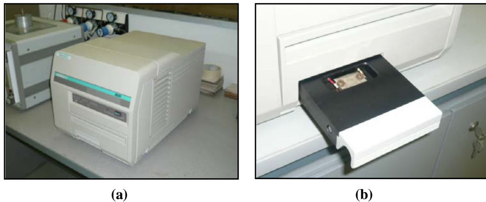
Figure 2: (a) Harshaw 3500 TLD reader and (b) planchet heating with read-out pan
