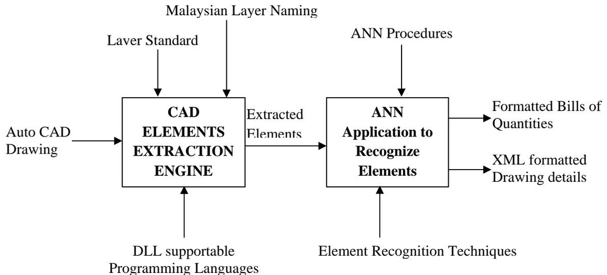
**Figure 2: Extraction Algorithm Process in IDEF0 Format**
