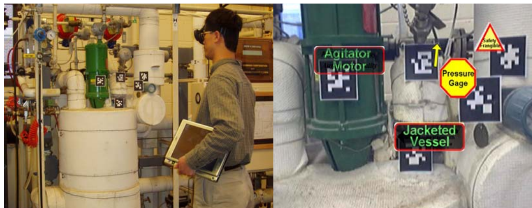
Figure 3. Illustration of User's Setup of AR EMS (Wang and Dunston 2006)
