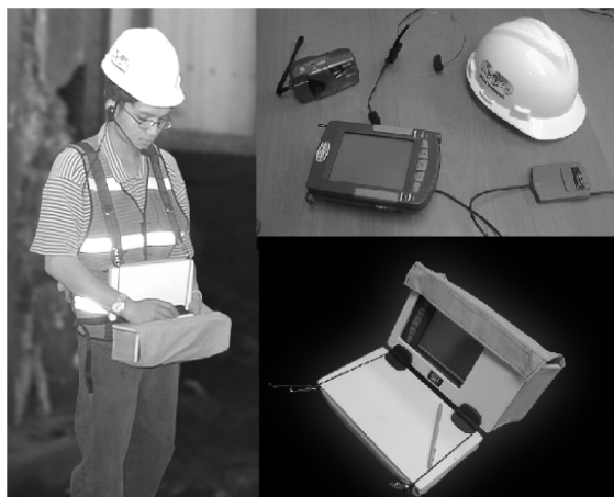
Figure 1. Illustration of Mobile Inspection Assistance (MIA) system (Sunkpho et al. 1998)
