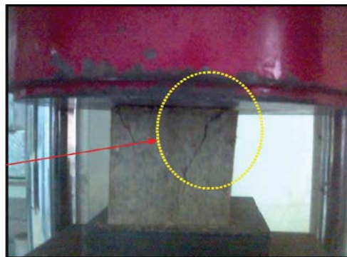
Figure 3: Tonipact machine for compression test of cube - The cube failure
