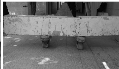
Figure 5: LFC Beam after Failure
