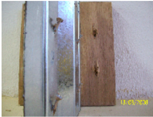
Figure 6: Sample Failure of Specimens - Slanted Screws
