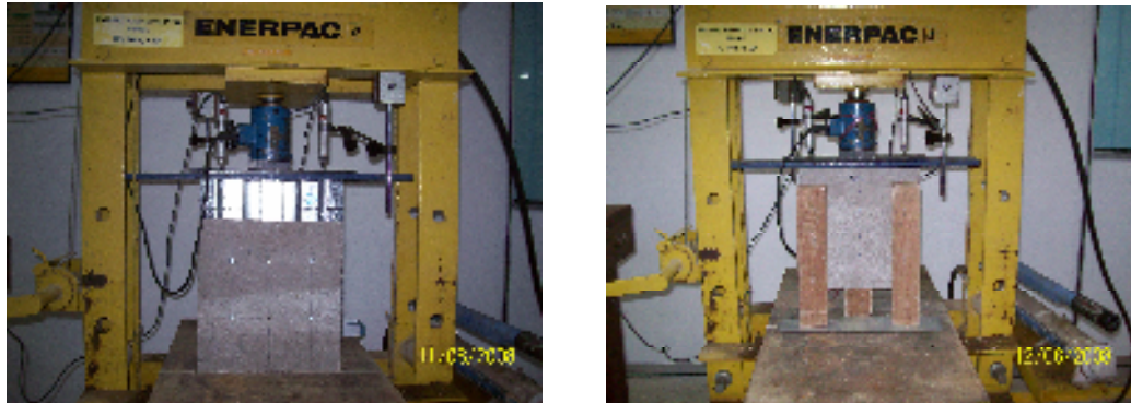
Figure 4: Specimens Testing of -(Left) Profiled Steel Sheetting and Dryboard, (Right) Dry Board and Timber
